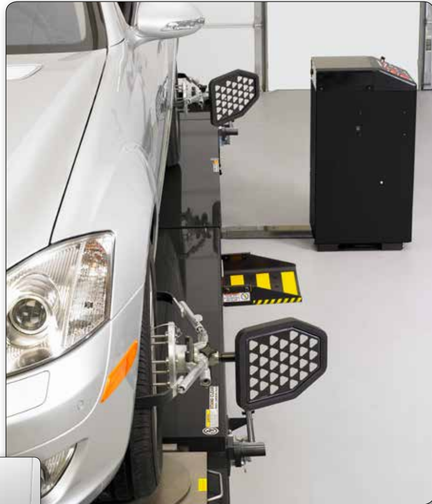
Lightweight, durable targets are easy to install.
