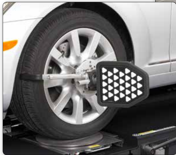
Targets contain no electronics to damage if dropped.
